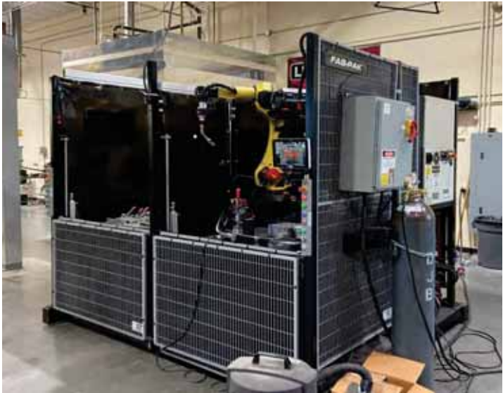
2 Bay Robotic Welding Cell
